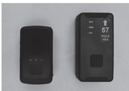
Figure 3. GPS trackers, compatible with 2G – left and 4G and 5G-right
